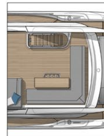
OPTIONAL FLYBRIDGE ARRANGEMENT WITH FIXED GRP SEATING AND TABLE
