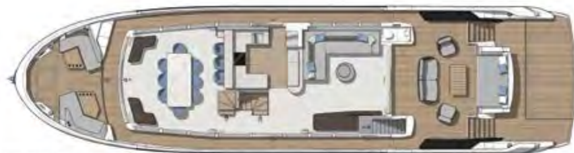
MAIN DECK – OPTION B - MID GALLEY WITH FORWARD DINING AND AFT SALOON Shown with optional twin anchor arrangement, side deck and foredeck decking, forward patio door, galley side deck door, dayhead and Sunseeker X-TEND™ transformer sunbead arrangement with loose cockpit furniture.
