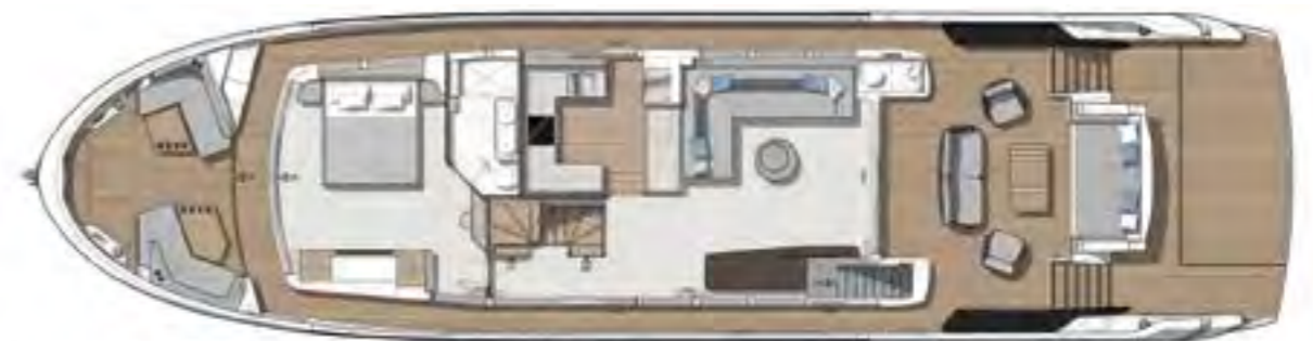
MAIN DECK – OPTION D - MAIN DECK STATEROOM WITH MID GALLEY AND AFT SALOON Shown with optional twin anchor arrangement, side deck and foredeck decking, forward patio door, galley side deck door, dayhead and Sunseeker X-TEND™ transformer sunbead arrangement with loose cockpit furniture
