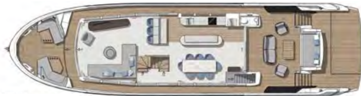
MAIN DECK Shown with optional twin anchor arrangement, side deck and foredeck decking, forward patio door, galley side deck door, dayhead and Sunseeker X-TEND™ transformer sunbead arrangement with loose cockpit furniture.
