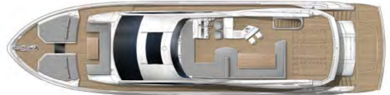
FLYBRIDGE Shown with optional coachroof skylight, flybridge teak decking, wetbar with raised shelf and 2 x bar stools
